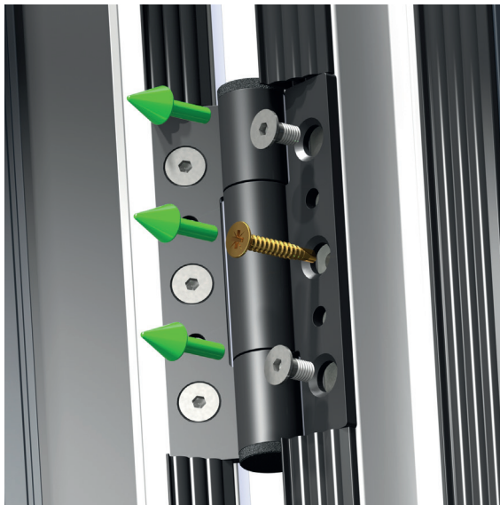
Removing these three screws for each hinge will allow the removal of the door sashes
