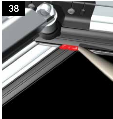
Now glaze the side frames before glazing the roof - this provides additional rigidity whilst working above. INSTALL TIE BARS(S) BEFORE GLAZING.
