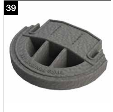
Take the 'soft touch' hub weathering shield. It fits by lifting the flaps on the ridge rain baffle to insert. NOTE: The weathering shield will need to be trimmed to suit to fit snugly. See p19/20 for trimming information.
