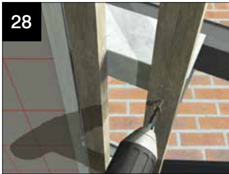
28 Fit second row of battens as described on page 40.
