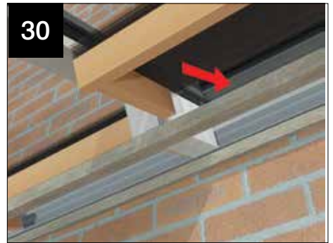
30 Slide remaining modesty panels into position, ensure that the batten on the screen is set 6mm back and screw fix to secure.
